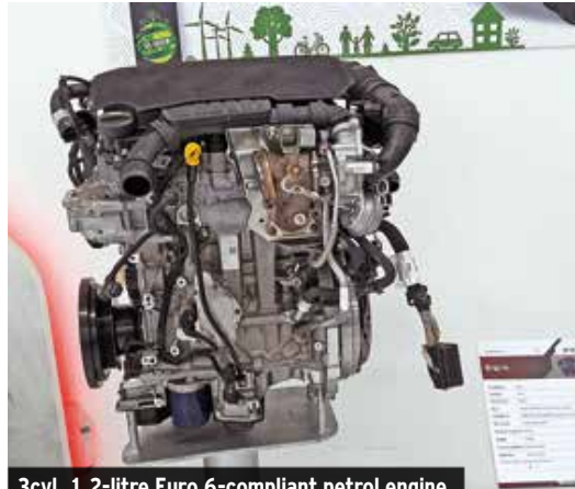
3cyl, 1.2-litre Euro 6-compliant petrol engine.
